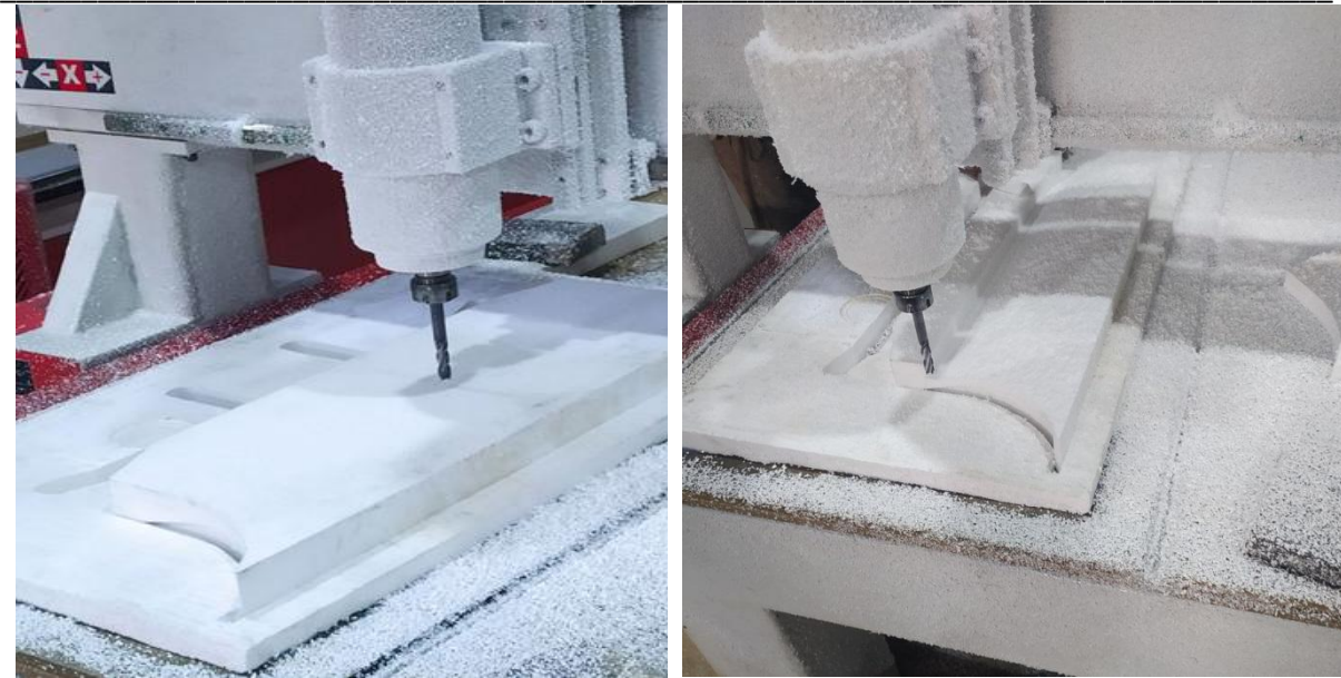
Figure 1. Machining process of the U-shaped sample on the “CNC ROUTER 2130” machine
