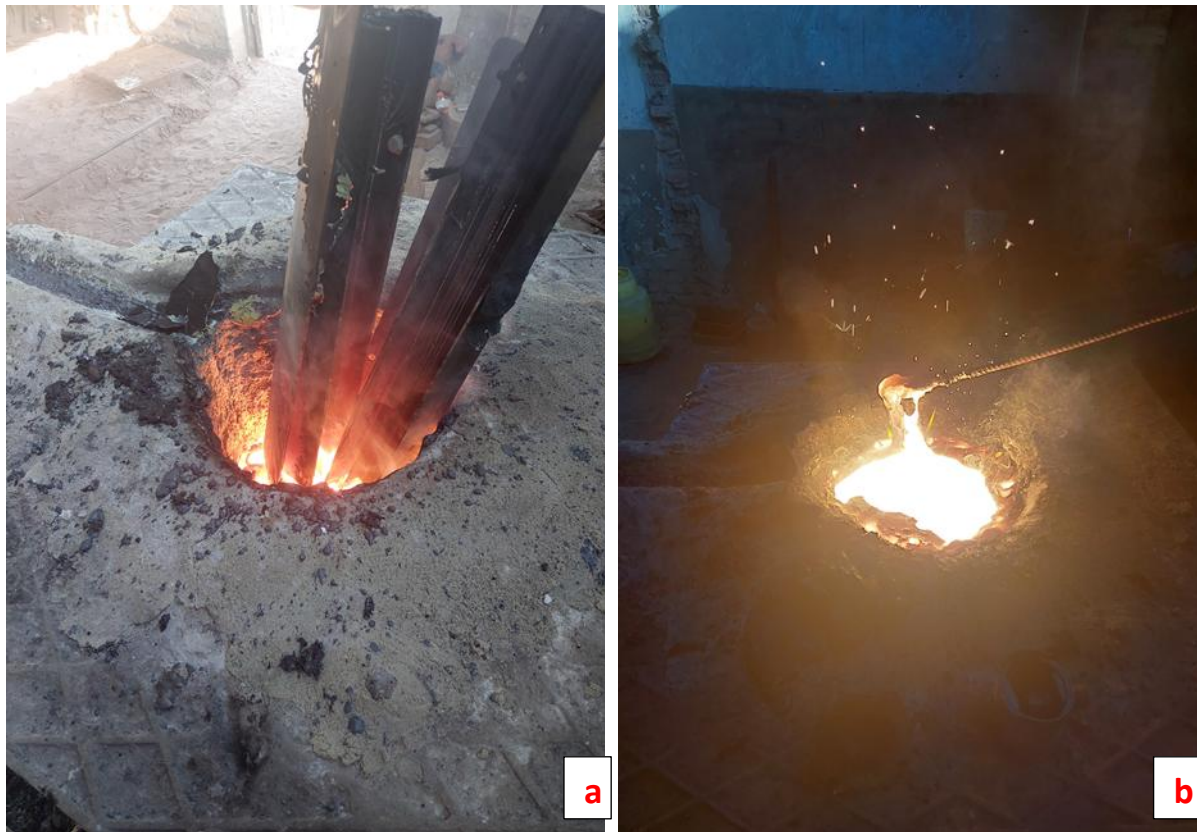
Figure 3. a) Melting process of the steel alloy in the induction furnace; b) Slag removal process from the molten metal
