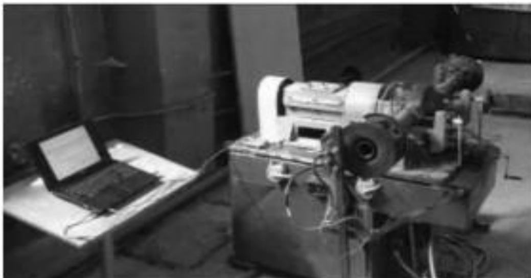
Figure 2. Stand for vibroacoustic diagnostics of drive axles of passenger cars
